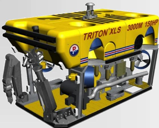
The Triton XLS system's 3,000 kg of through-frame lift provides a platform for a wide variety of tooling modules and custom intervention work skids.
